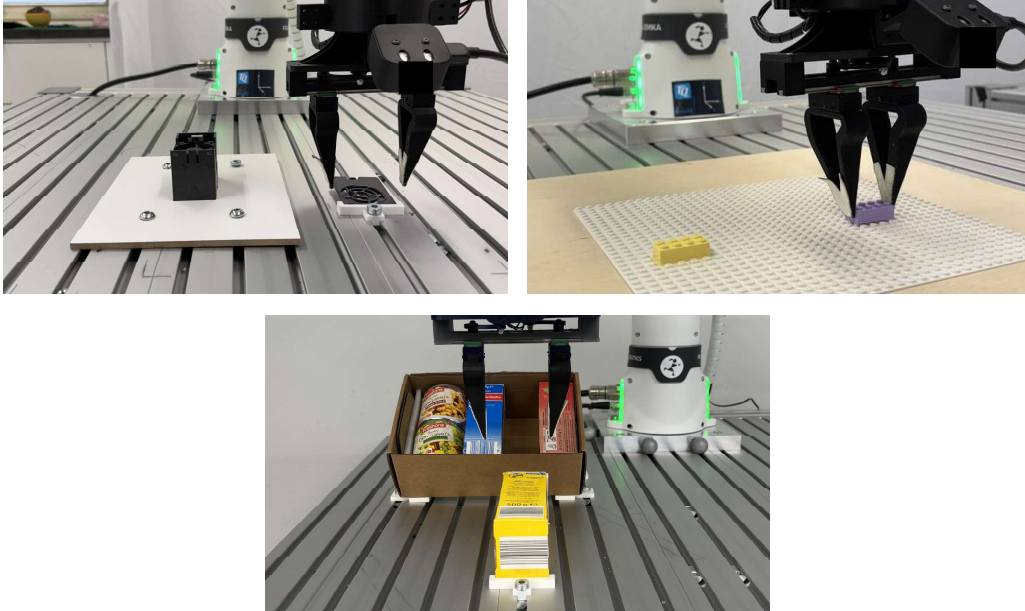
Figure 5: Data collection setups for our different scenes. Our setup requires a fixed scene for data collection. For Lego, we use the base plate to define the layout. For the other tasks, we 3D print small fixtures to keep the part in place.
