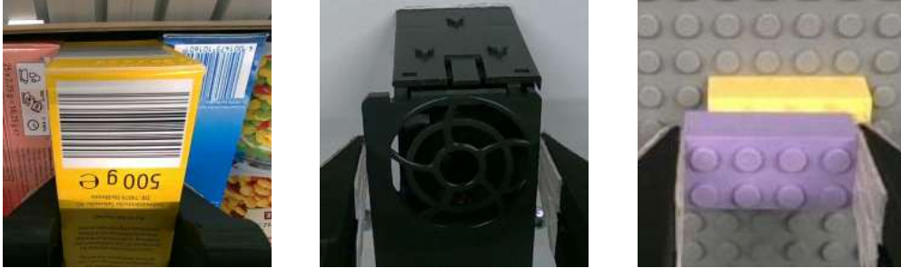
Figure 11: Visual inputs used for our policies. Policies for our method receive a single viewpoint from a wrist-mounted camera as input that is cropped to the critical insertion region of the task.
